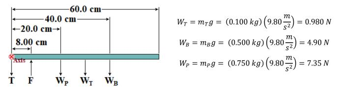
Setting the sum of forces equal to zero will give us 1 equation with 2 unknowns. Consequently we will need to use a torque equation.
