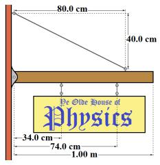
**Example**: A 2.50 kg sign is hung from an 11.0 kg beam as shown in the diagram. The sign is balanced so that half its weight is supported by each of the two wires above it. The beam is attached to the wall on the left by a frictionless pin that allows it to rotate and held in place by a guy wire above it. Determine the tension in the guy wire.
